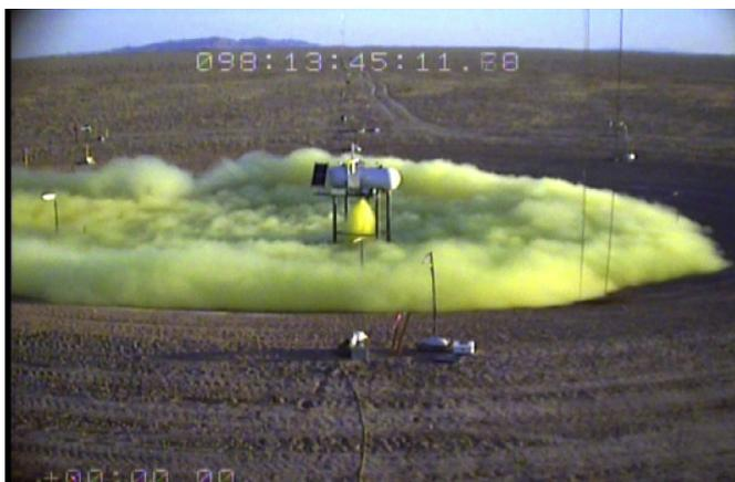
Fig. 1. JR I Trial 2 at 22 s. One ton chlorine release with  $u = 0.6$  m/s.
