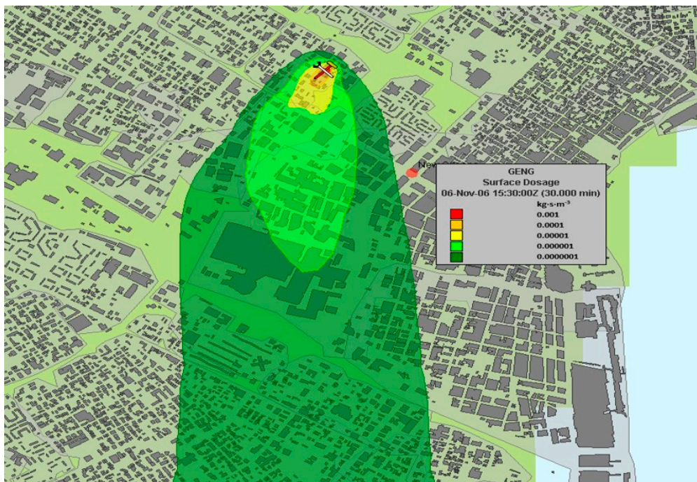
Figure 1. Example of urban dispersion prediction provided by Urban Dispersion Model (UDM). Colour contours show downwind dispersion of plume through the urban environment. From Herring, S. and Huq, P., 2016, 17th International Conference on Harmonisation within Atmospheric Dispersion Modelling for Regulatory Purposes [7].
