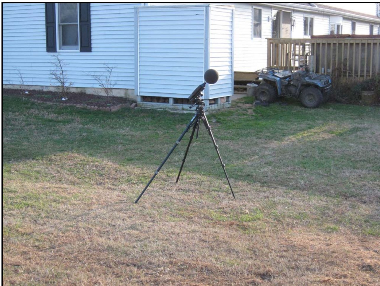
View of the tripod-mounted CEL 593 sound analyzer and wind screen in the back yard of the 16 Hoornkill Avenue property looking toward the house.
