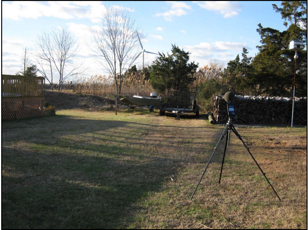
View of the tripod-mounted CEL 593 sound analyzer and wind screen in the back yard of the 16 Hoornkill Avenue property looking northwest toward the UD-Gamesa wind turbine (approximately 2,200 feet in the distance).
